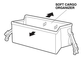
2. Attach the two partitions to the soft cargo organizer by connecting the inner snaps.
