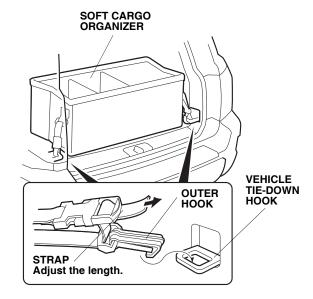
4. Adjust the length of the straps as needed to secure the organizer to the tie-down hooks.
