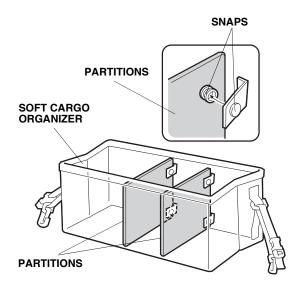
3. Place the organizer in the cargo area of the vehicle, and attach the outer hooks on the organizer to the vehicle tie-down hooks.
